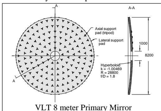
The 23 tons VLT primary mirrors are in Zerodur produced by Schott Mainz (Germany).
