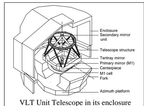
**The VLT M1 mirrors optical specifications :** The optical figuring specifications of the VLT primary mirrors take into account the presence of an active mirror support and the effects of atmospheric turbulence. REOSC shall therefore use the active support during final tests within a limit of  $\pm 120$  N to remove some low spatial frequency figuring errors. In addition, the first three natural modes are limited in peak-to-valley amplitude.
