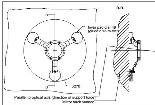
REOSC optimized, in cooperation with ESO, the interface between the axial actuators and the mirror blank. This is a tripod assembly which, by inducing local bending moments, reduces by a factor 3, down to 16 nm RMS, the 50 nm RMS wavefront high spatial frequency print through obtained otherwise with a simple point like support.
