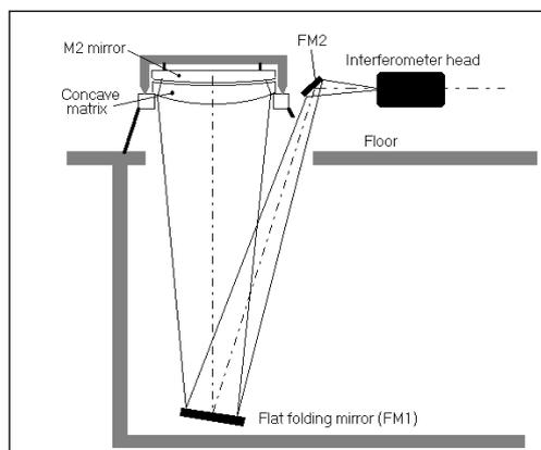
**The optical test set-up** A full pupil optical test set-up was designed and built to test the convex aspherical surface. As shown on the sketch this was done with a 1250-mm diameter Zerodur matrix being the exact negative of the mirror. The fringe pattern is collected by the rear side of the matrix towards the interferometer head at 14 meter distance.
