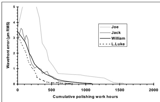
**Convergence upon polishing** Once transferred to the polishing machine, polishing was performed with minimum figure loss and final figuring conducted to reach the optical specifications. Again Joe was the pathfinder perturbed by the non uniform angular distribution of the lateral pads that generates some astigmatism.
