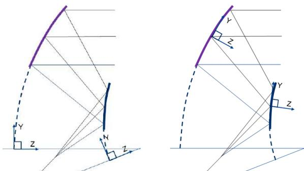
Figure 6. Main optical referential + Tilts & Decenters versus individual referential per mirror
