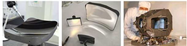
Figure 7. JWST NIRSpec optics, conventional off-axis
