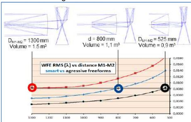
Figure 1. Pleiades WFE RMS vs  $D_{M1-M2}$  and freeform
