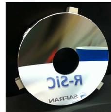
Figure 10. R-SiC demonstration on 20-cm mirror
