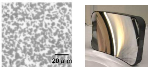
Figure 9. SiC is porous and needs a polishing layer
