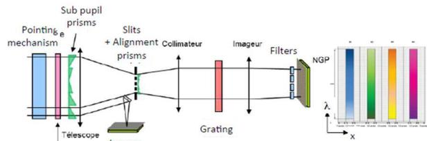
Figure 4. MicroCarb multiband spectrometer concept
