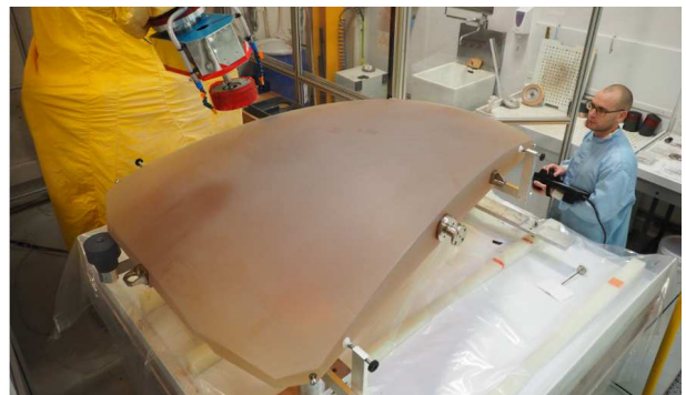
Figure 12. The M2 sector aspheric reference plate installed for first robotic lapping cycles.
